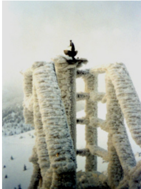
Heliograph covered with hoar-frost (heliograph measures sunshine duration)
